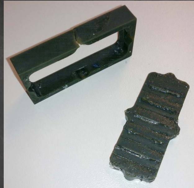
Adhesion between mold and chip ( Aureus from VDM, DLP Printing)
